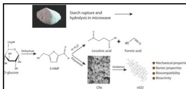
Figure 1. Transformation of starch to nGO
